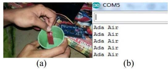
Gambar 15.(a) Uji coba sensor air terhadap air, (b) Tampilan sensor air di Arduino IDE
