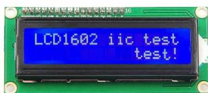
Figure 4. LCD 16 x 2 I2C
