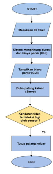
Figure 9. Flowchart vehicle exit process
