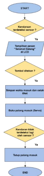
Figure 8. Flowchart vehicle entry process
