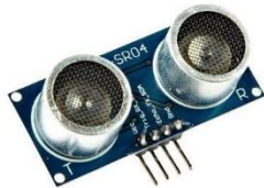
Figure 2. Ultrasonic Sensor HC-SR04
