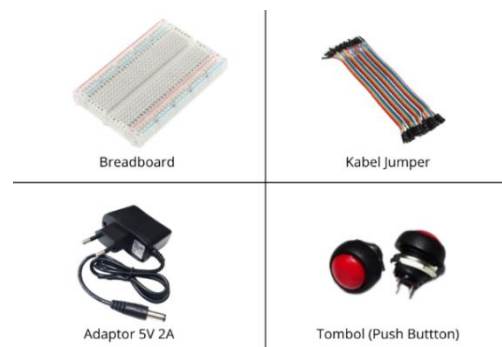
figure 6. Supporting tools used: breadboard, jumper cable, adaptor 5 V 2 A, and input button (push button)
