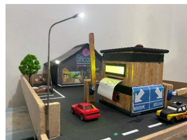
Figure 11. The vehicle is detected by the sensor upon entry and the system automatically prints a ticket.
