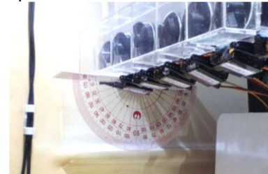
Figure 14. Testing of the Herbal Powder Valve in the Vending Machine
