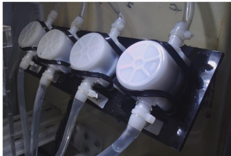
Figure 13. Water Flow Sensor YF-S401 for Vending Machine
