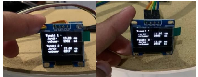
Figure 10. Liquid Surface Distance Display on Tank Read by Ultrasonic Sensor
