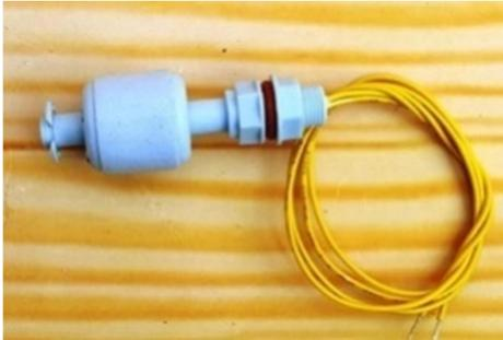
Gambar 7 Water level float switch
