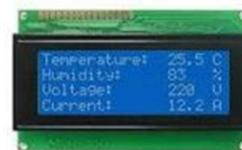
Gambar 9. Liquid Crystal Display
