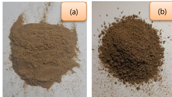
Figure 1. Water hyacinth powder: (a) before, and (b) after NaOH activation
