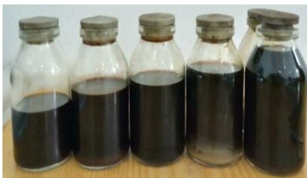
Figure 3. Pyrolysis Liquid Before Distilling
