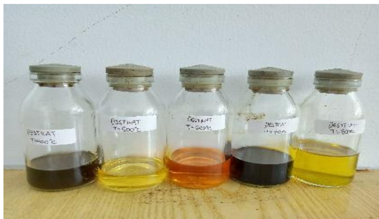
Figure 5. Pyrolysis Fuel from All Temperature Variations
