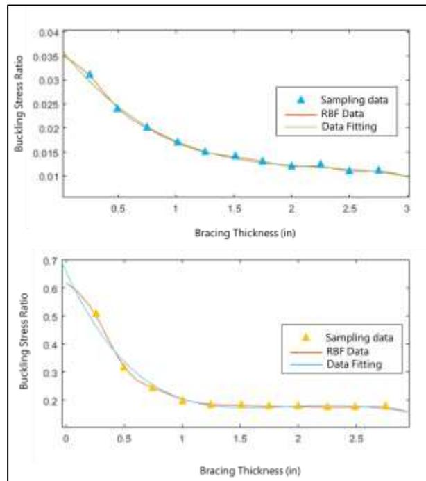
Figure 6. The variations of UC Ratio with Bracing Thickness Based on RBF Model
