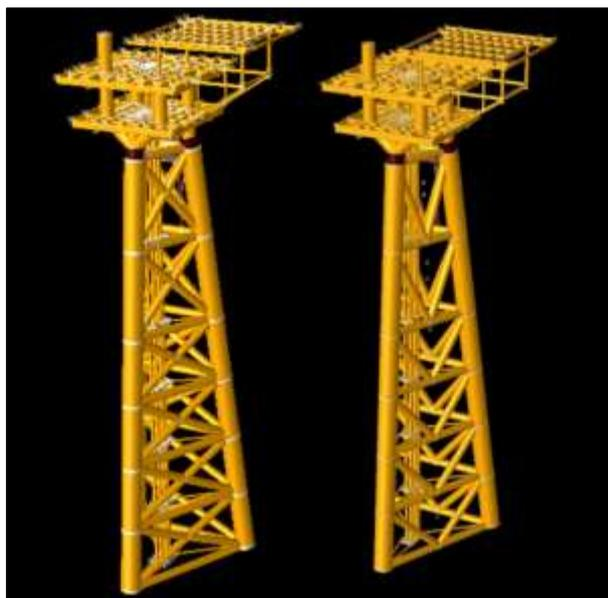
Figure 1. Jacket Structure Modelling with X-type bracing (left) and V-type bracing (right)
