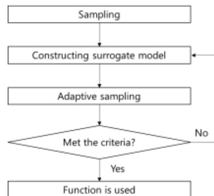
Figure 2. Process of Constructing a Surrogate Model
