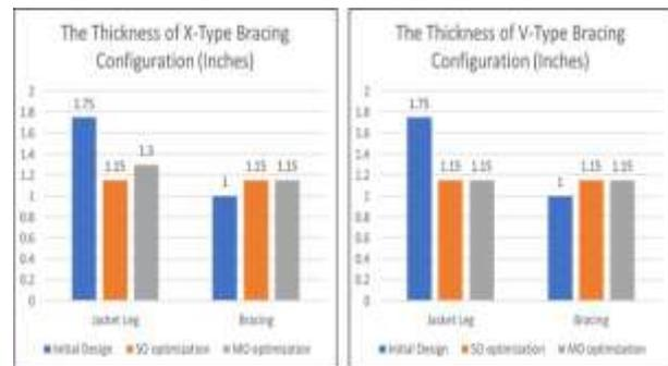
Figure 8. The Thickness of Tubular Members in The Initial And Optimum Designs Of The Jacket Platform
