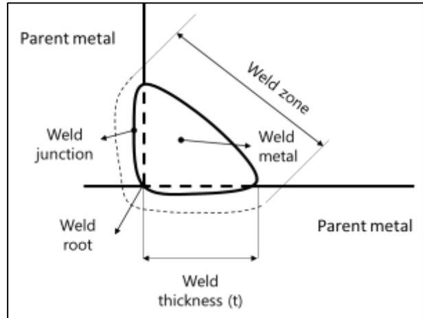
Figure 4. Weld Illustration of Tubular Joint (AWS D1.1, 2010)
