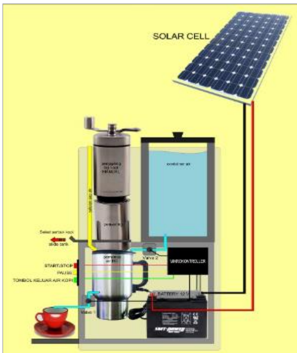
Gambar 2. Desain Perancangan Mesin Grinder Coffee Brewer Berbasis Photovoltaic
