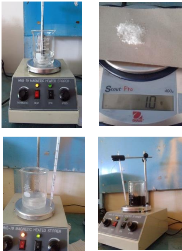
Figure 1. Mixing Activated carbon, binder, and PVA
