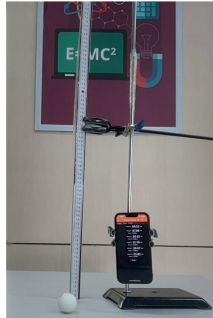
Figure 1. The materials are readily available in a standard Physics Laboratory like retort stand, meter ruler, clamp, and with addition of smartphone's PhyPhox application.
