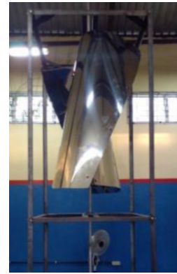
Fig. 1. Construction of a helical savonius windmill.
