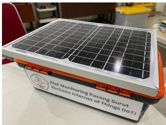
Gambar 6. Desain Alat Monitoring Pasang Surut
