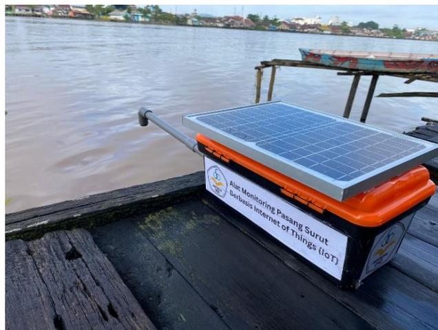
Gambar 12. Ujicoba lapangan alat monitoring pasang surut
