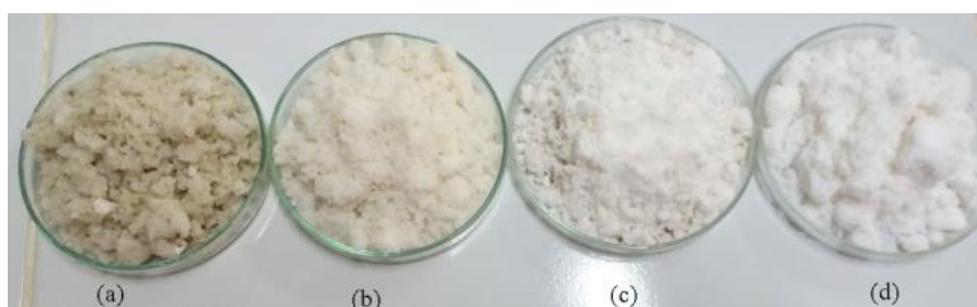
Figure 7. Comparison of salt appearance: (a) crude salt; (b) 1 st purification; (c) 2 nd purification and (d) 3 rd purification
