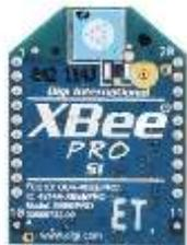
Gambar 4. Modul *wireless* XBee-PRO[5]
