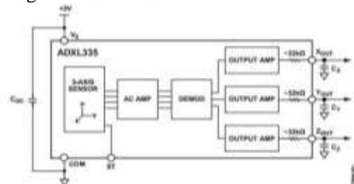
**Gambar 3.** Accelerometer ADXL335[1]
