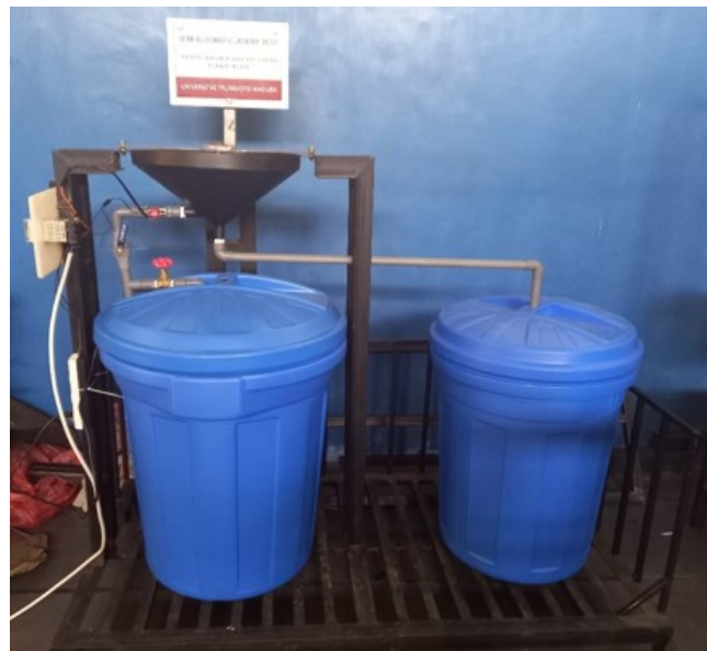
Figure 7. Semi Automatic Jominy Test Tool Design Results
