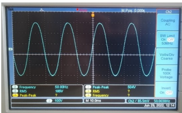
Figure 8. Result of output inverter with bulb load
