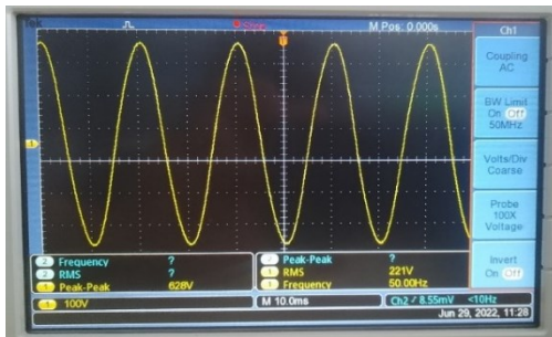
Figure 7. Sinusoidal waveform from inverter output (with passive filter and transformer)
