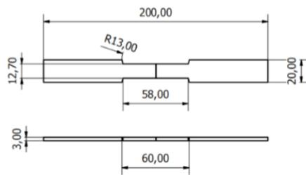
**Figure 1.** Design of the specimen (in mm) based ASTM A370
