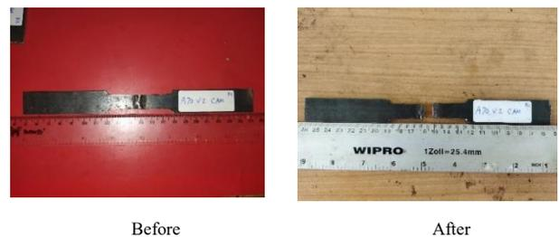
**Figure 2.** Specimen before and after tensile test
