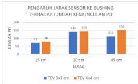
Figure 10. Graph of the number of PDs at 8kV level
