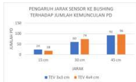
Figure 8. Graph of the number of PDs at 6kV level
