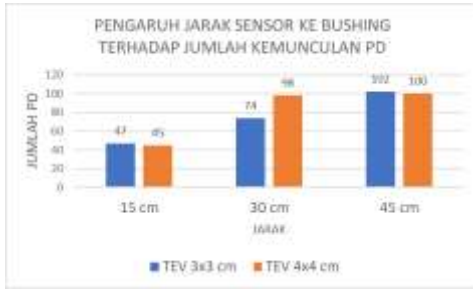
Figure 9. Graph of the number of PDs at 7kV level
