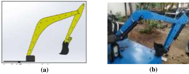
Figure 7. (a) Design Arm Backhoe; (b) Prototype Arm Backhoe.
