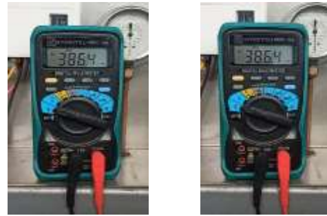
Figure 5. Voltage Measurement on (a) Cutting Motor; (b) Condenser.
