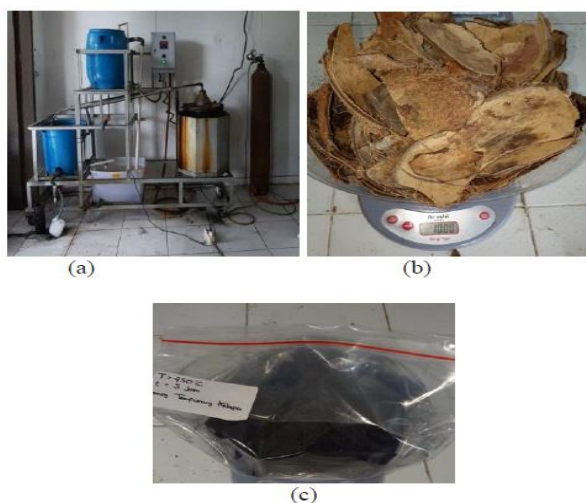
Figure 1 (a) pyrolysis equipment; (b) coconut shell bunches; (c) coconut shell charcoal.
