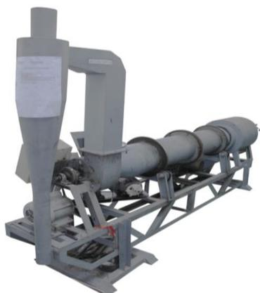
Gambar 2 rotary dryer
